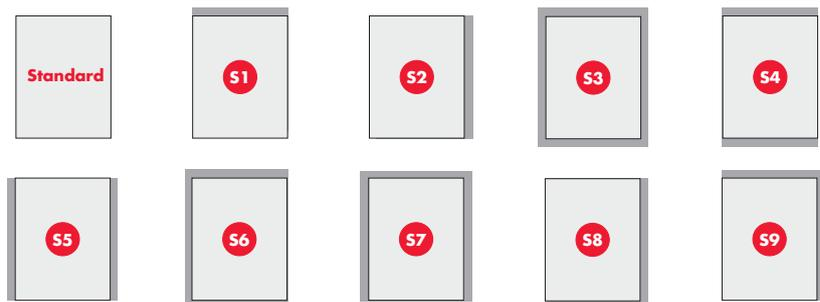
Overlap of the facing is about 30 mm. Overlap measure can vary in special dimensions and if needed for special purposes.
